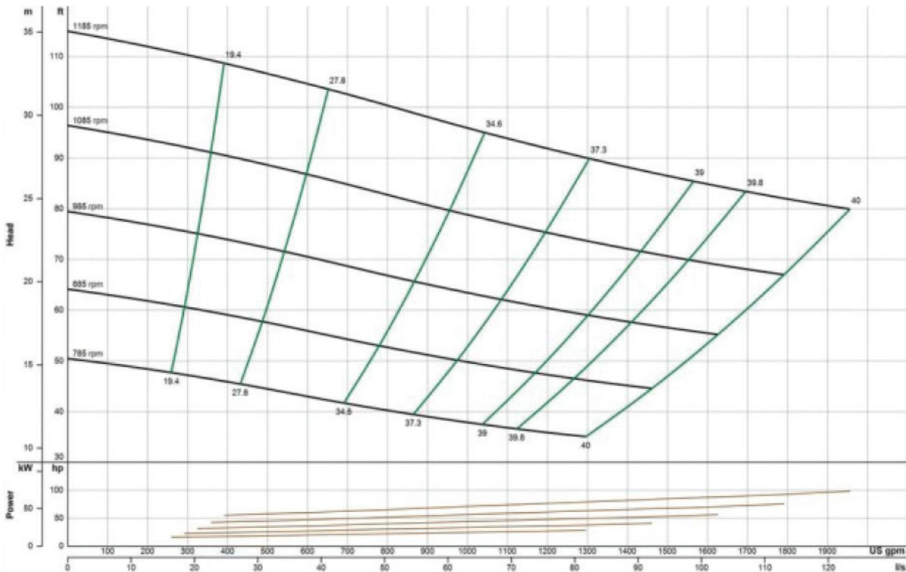
\*General pump curve based on water at 1200 RPM. Contact us with your specific material for a custom pump curve.
