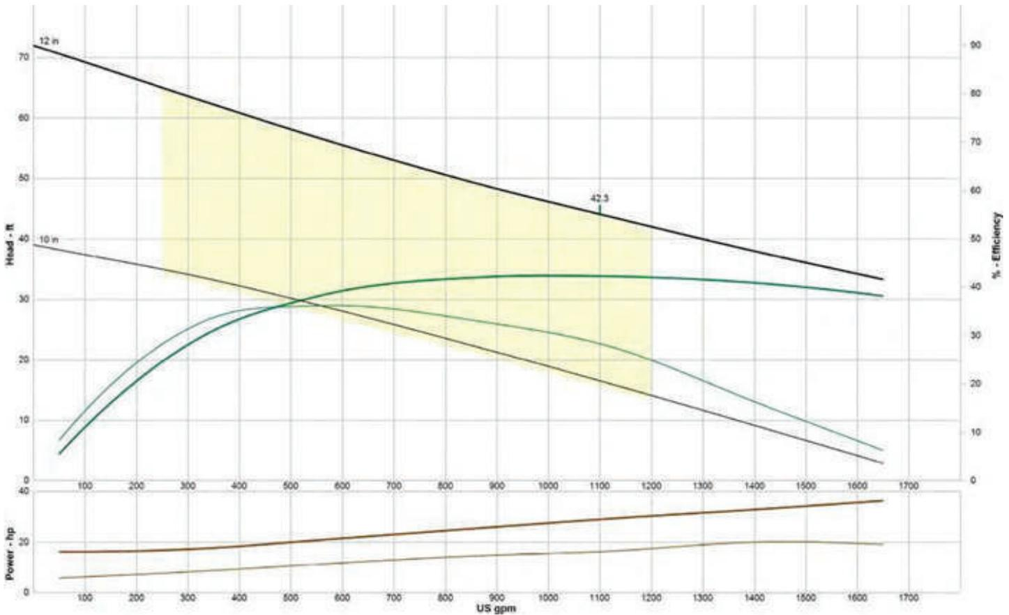
\*General pump curve based on water at 1200 RPM. Contact us with your specific material for a custom pump curve.
