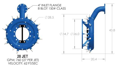
\*\*GPM & VELOCITY CALCULATION BASED ON 4" CENTRIFUGAL WATER PUMP, 760 GPM WITH 81' HEAD
