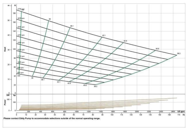
\*General pump curve based on water with 900 RPM motor. Contact us with your specific material for a custom pump curve.
