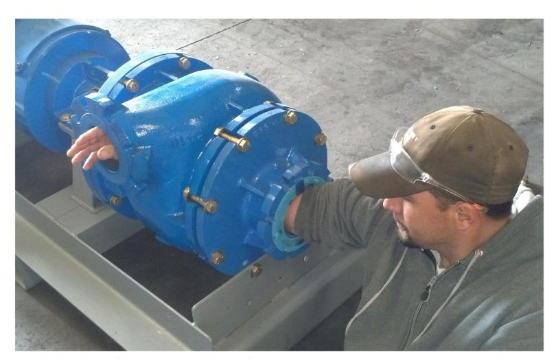
4-Inch fully intact Eddy Pump with enough tolerance for an arm to go through the intake and out the discharge
