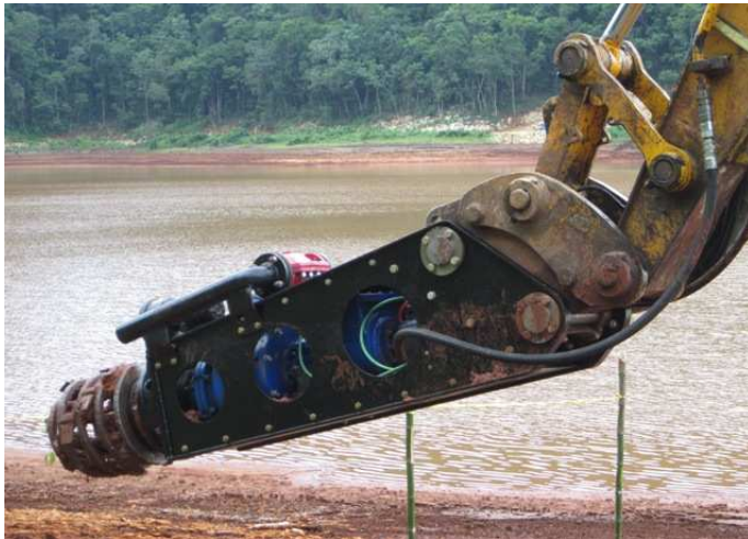
PHOTO 3.1: Eddy Pump in Excavator Attachment
