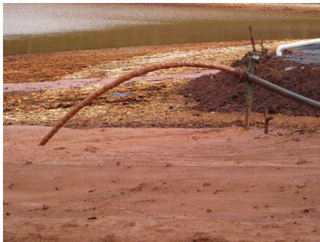
Photo 5.3: Mud pump in re-circ / priming mode Photo 5.4: Discharge of muds ( \pm 30 l/s, \pm 37\% solids)
