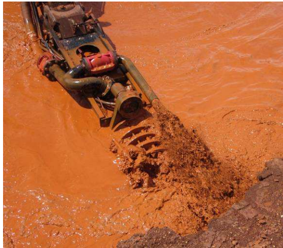
Photo 5.3: Mud pump in re-circ / priming mode Photo 5.4: Discharge of muds ( \pm 30 l/s, \pm 37\% solids)
