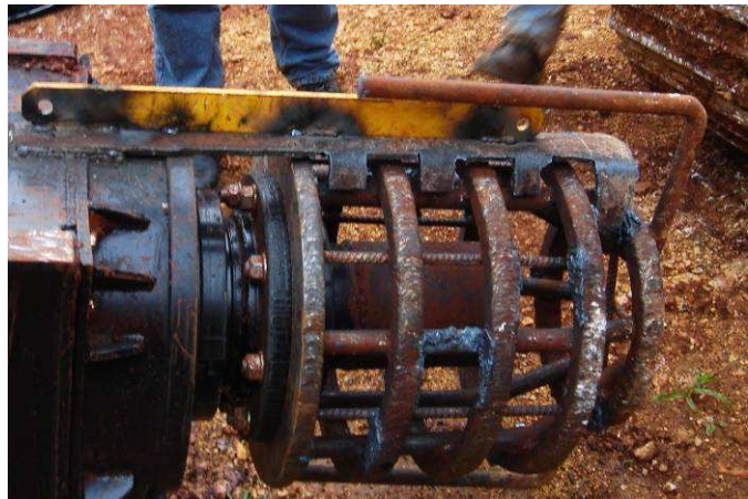
Photo 5.2: Cutter Head With Comb added
