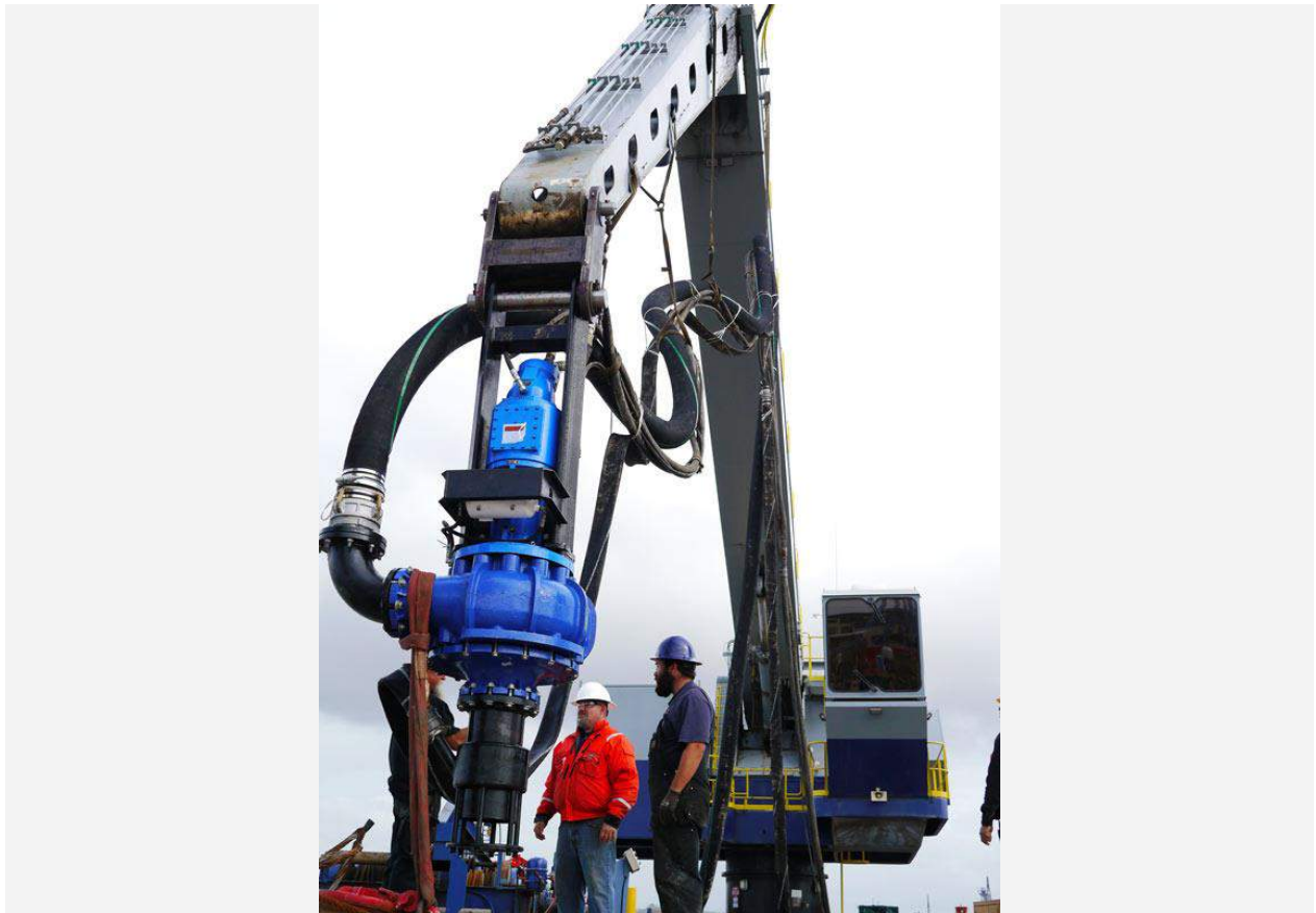
8-inch Slurry Pump with Jetting Ring. Cable or boom mount options. 2017 Project.
