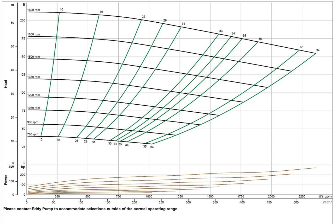
\*General pump curve based on water with 1800 RPM motor. Contact us with your specific material for a custom pump curve.
