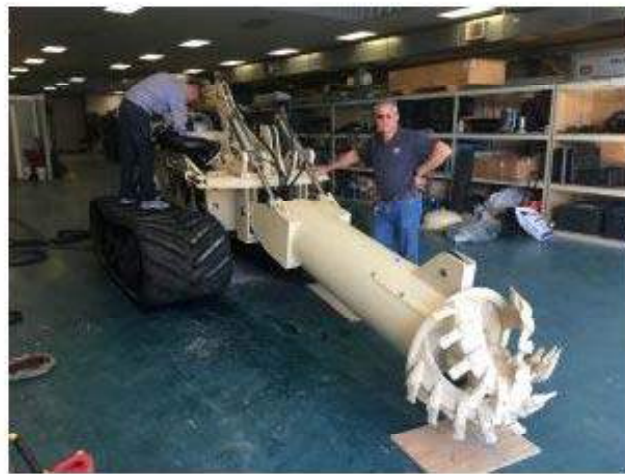
A close up of the cutter head that can be used on the MRSD as an alternative head.
